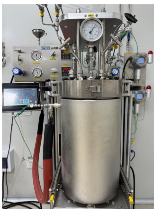
Fig. 2 Dynamic high heat oxygen partial pressure accelerated aging device.
